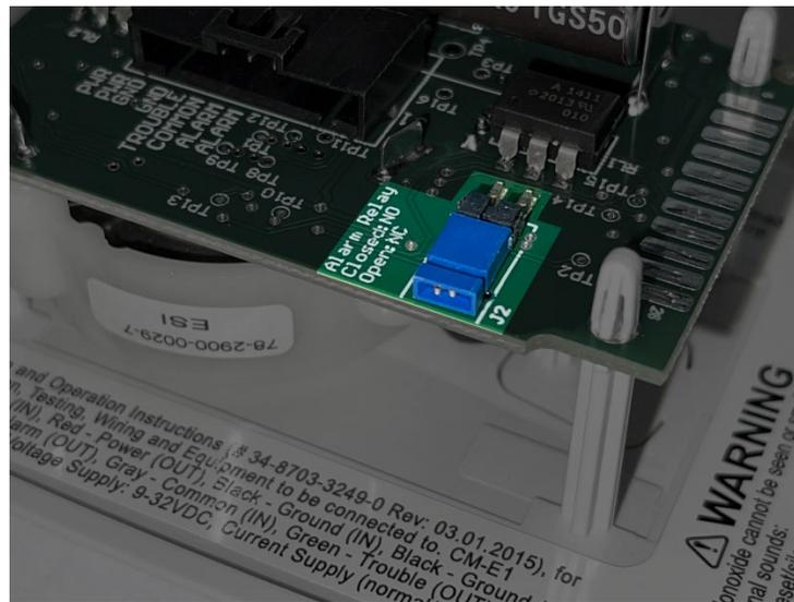
Figure 3-6 – Alarm Relay Jumper J2 Location
